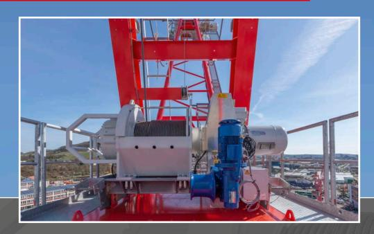
A maintenance-free multi-disk secondary brake on the luffing winch is included as standard and available as an option for the hoisting winch.
